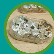
Disconnect and tape all tabs to protect terminals
